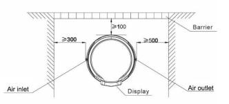
The Evo 270 is designed for external installation; however, if possible, installing the system under the house eaves or in a sheltered environment may help prolong the life of the system.
